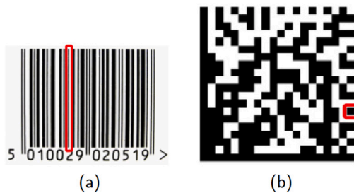
Fig. 2. (a) shows an element (or module) of a linear barcode, while (b) shows an element (or module) of a 2D barcode.
