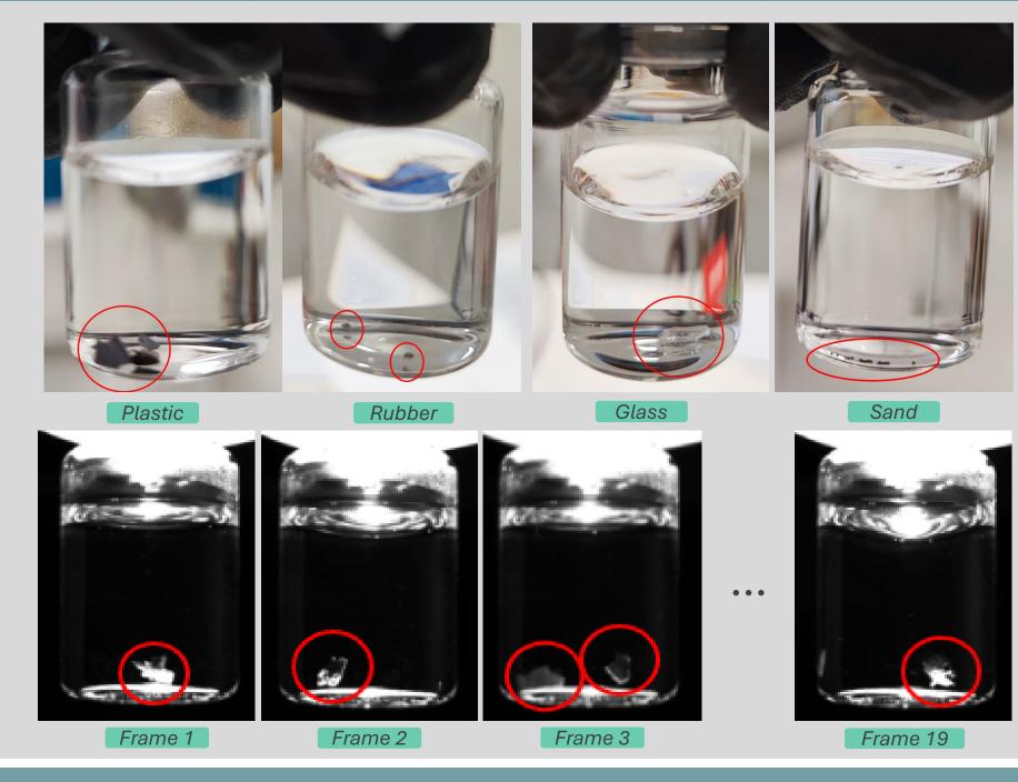
The dataset was acquired internally by *Performing Beyond Limits (PBL)* and consists of 2,426 vial sequences filled with water, with 19 frames each. It includes five different classes: one represents the absence of impurities, while the others correspond to four foreign particles: burnt plastic, rubber particulates, glass fragments, and sand debris.
