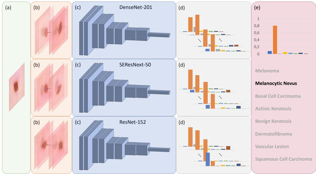
**Fig. 6:** Illustration of the proposed ensemble method. Given an input image (a) at inference time, multiple versions of it are obtained by means of random data augmentation. Augmented images (b) are then fed to a CNN (c) and calibrated outputs (d) are obtained. This process is repeated over multiple CNNs and, finally, all of the network outputs are averaged together in the last step in order to obtain the final prediction (e).
